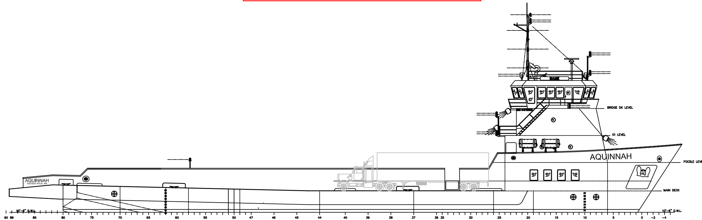
AQUINNAH OUTBOARD PROFILE @ 235' LOA WL LENGTH @ 10'-6" DRAFT= 199'-10"
